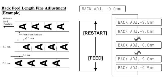
NOTE: The fine adjustment value equals the sum of the fine adjustment values set by the PC command and this parameter. The maximum back feed lengthfine adjustment value is ±9.5mm. When the value reaches the maximum, the value remains unchanged even if the subsequent fine adjustment is performed.
